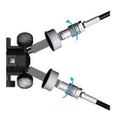
**a.** To depressurise both systems simultaneously, open both control valves and gently open the release valve by rotating the release knob anticlockwise.
