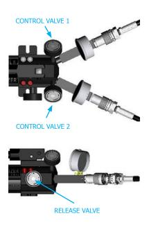
**a.** If control valves 1 and 2 are set to the fully open position and the release valve is screwed fully, when the pump handle is raised and lowered both hydraulic systems will be pressurised to an equal pressure (max. 700 bar (10 000 psi)).
