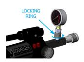
2. Ensure the hydraulic system you wish to pressurise has been bled and is free from air and leaks. Connect the pump into the system using the screw connector supplied with the pump, push the male and female connectors together fully and rotate the locking ring clockwise until fully tight.
